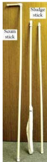
This process is to determine the distance between the bottom of the scum layer and the bottom of the outlet baffle or tee.
