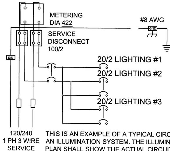
THIS IS AN EXAMPLE OF A TYPICAL CIRCUIT FOR AN ILLUMINATION SYSTEM. THE ILLUMINATION PLAN SHALL SHOW THE ACTUAL CIRCUIT AND WILL BE REVIEWED AND APPROVED BY THE COUNTY ENGINEER.
