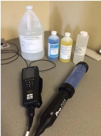
Figure 5 – YSI ProDSS Sonde with calibration solutions
