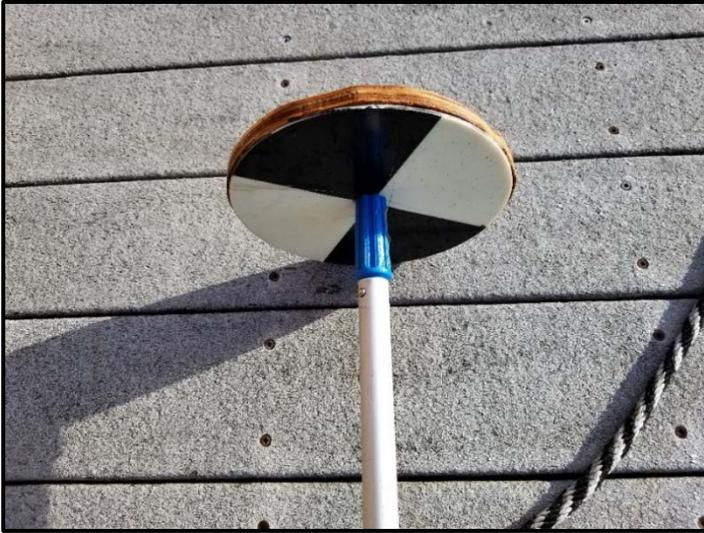
*Secchi disk adhered to base and telescoping pole*
