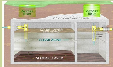
The first basic part of the O&M inspection is the monitoring of the layers of scum and sludge inside the septic tank (see brochure titled “Is It Time to Pump” for more information.) This simple monitoring and timely pumping can greatly extend the life of your system.
